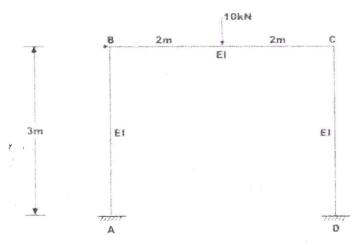
Q.6 Analyse the rigid frame shown in figure below by moment-distribution method. Moment of inertia of different members is shown in the diagram. (08)
