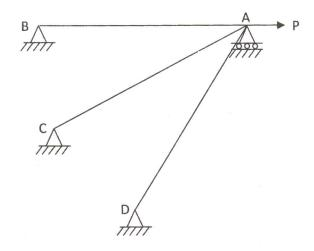
Q.5 Analyse the rigid frame as shown in Figure below using slope deflection method. Assume *EI* to be constant for all members. Draw bending moment diagram and sketch deflected shape. (08)
