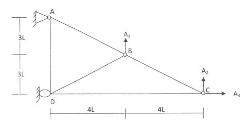
Q.2 Analyse the frame shown in Fig. below using flexibility method considering only flexural deformations. The flexural rigidity EI is the same for all members. (10)
