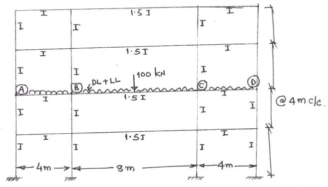
Loading on beam ABCD is, DL = 25 kN/m & LL = 20 kN/m. Design the beam section at support at B, if the moment due seismic is  $\pm$  90 kN.m . The worst combination of loads should be considered for design and relevant provisions of Indian codes.
