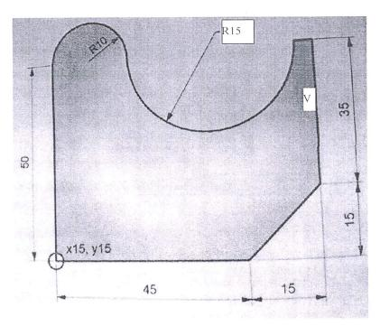
**b.** Following component is to be made using CNC Turning Center equipped with FANUC controller. Write a NC part program using Turning FACING cycle. Assume workpiece material as MS and Cutting tool material as HSS.
