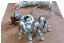
Robotic Tentacle arm using multiplexer
