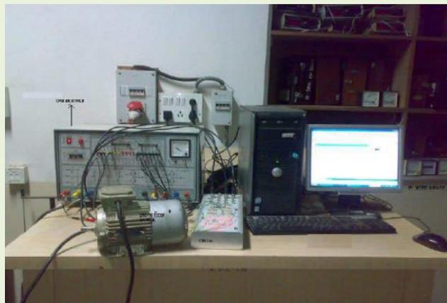
**Experimental setup for validation of SVM-DTC control algorithms**
