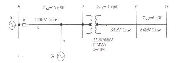
Q.3 For the radial distribution system shown in the diagram, coordinate the IDMT over (9) current relays  $R_1$ ,  $R_2$  and  $R_3$  using the data in Table 1. Use IEC standard inverse characteristics.
