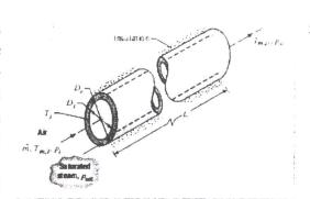
a temperature of  $T_{m,i}$ =17 °C, and a flow rate of 0.03 m/s, while saturated steam at 2.455 bars condenses on the outer surface of the tube. If the length of the annulus is L=5 m, what are the outlet temperature  $T_{m,o}$  and pressure  $p_o$  of the air? What is the mass rate at which condensate leaves the annulus?
