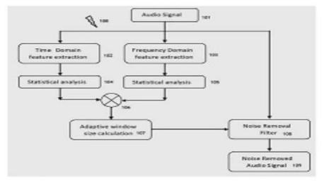
Figure 1. System architecture of dynamic time and frequency domain approach for removing noise
