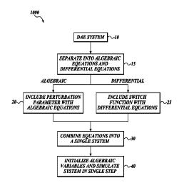
method includes generating a model of the rechargeable battery; determining one or more initial conditions for one or more algebraic variables of the model using a solver; holding differential variables of the model static by a switch function while determining the one or more initial conditions; applying the initial conditions to the model by the switch function; and determining one or more parameters for the rechargeable battery by solving the algebraic and differential equations.
