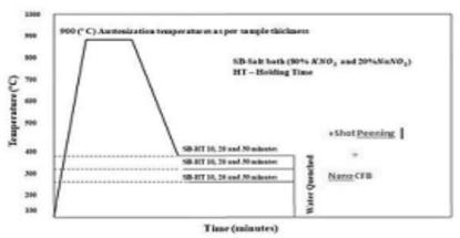
Figure 1. Heat treatment cycle used in present work
